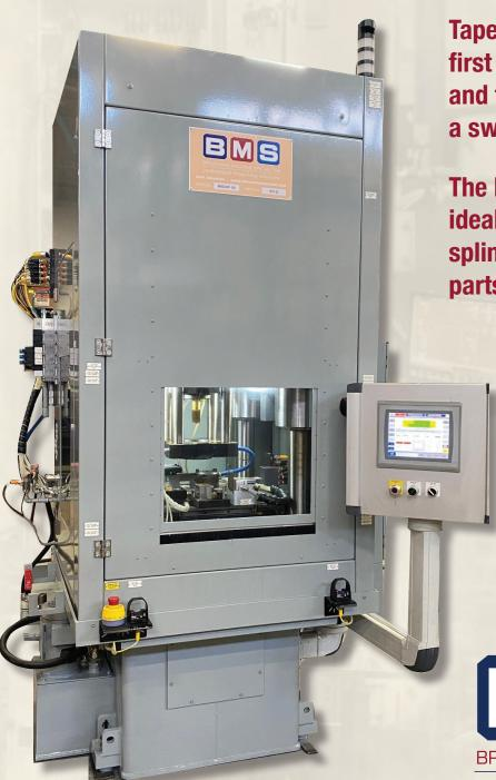
Tapered splines are created by first broaching a straight spline and then tapering the spline using a swaging process.
